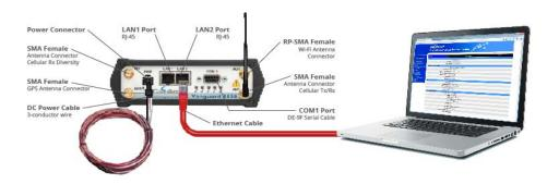
**Step 5** Connect the DC power cable (or optional AC power adapter) to an applicable power source and plug the connector into the modem. If using the fused power cable to connect to a DC supply (car battery), use the following diagram and pin-out table to connect the unit.
