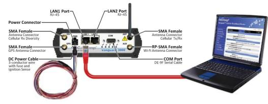
**Step 5** Connect the DC power cable (or optional AC power adapter) to an applicable power source and plug the connector into the modem. If using the fused power cable to connect to a DC supply (car battery), use the following diagram and pin-out table to connect the unit.
