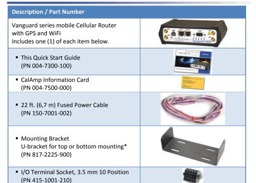
\* U-bracket includes four #8-32 × ½ (3/8-inch tread length) black plated stainless steel slotted hex flange cap screws to fasten the bracket to the sides of the Vanguard chassis.
