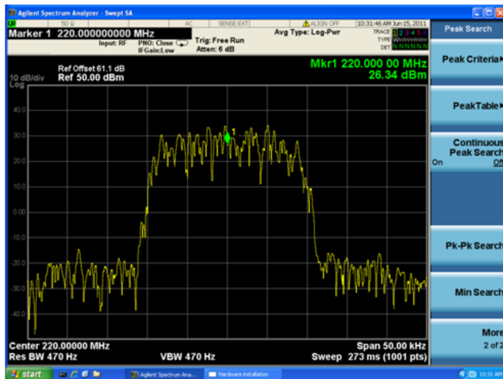
Figure 26 Typical transmission spectrum (DQPSK)
